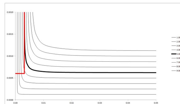
**Figure 4:** A sample analytic solution for the streamlines along and inside the jet. Note that the top electrode here is outlined in red, and that the centerline of the jet lies on the line  $y=0$
