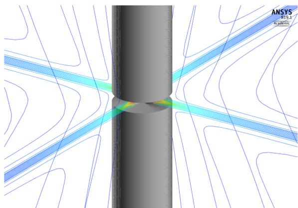
**Figure 2:** 3D diagram showing streamlines of the arc jet as well as streamlines of the ambient gas being entrained by the jet.
