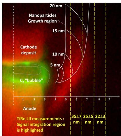
**Figure 1:** Experimental data [1] showing the arc region as well as the region where the majority of nanomaterial formation occurs. Note that this is experimental data, and therefore convection, outlet placement, and other factors break the top-bottom symmetry seen in other figures.
